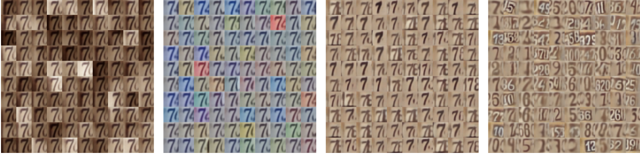
Figure 4. Hierarchical sampling on SVHN. Left: The latent code at bottom layer ( z_1 ) represents the background light and shading. Center-left: the latent code at second bottom layer ( z_2 ) represents the color schemes. Center-right: the latent code at second top layer ( z_3 ) encodes the shape variations of the same digit. Right: the latent code at top layer ( z_4 ) captures the digit identity and the general structure.
